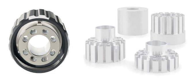
The outer contact modules shell is a CrossTalk-proof section dedicated to signals that are particularly sensitive to interference and cross-talk phenomena, such as ethernet lines and digital signals in general. The central insert is an electrically insulated section for signal types requiring high insulation between contacts, such as main power, speaker lines or analog audio signals.
