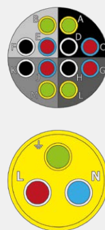
Central insert male Wiring diagram SGH 8.1 | SGH 16.1
