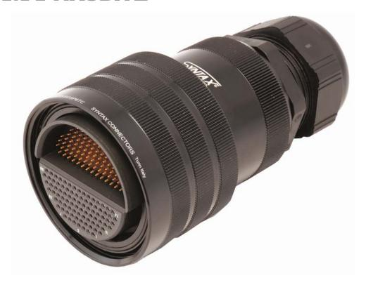
The SYNTAX® SMA connectors are configured in the 122 pins for multicore cables until 40 pairs and 176 pins for multicore cables until 58 pairs and are fully compatible with the existing fixed pin solder type & crimp type MASS connectors, and use the same inline and panel mount housings.
