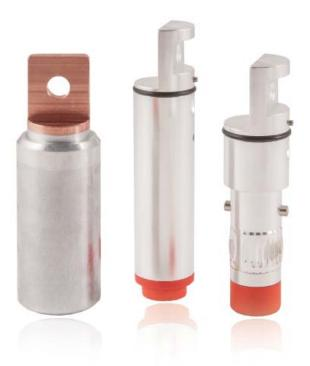
SPY EasiLUG is a quick, safe and easy means to fit lug terminal single core aluminium or copper cables into a classical Power Syntax<sup>®</sup> single pole connector. It combines the reliability of a lug termination cable with the convenience of a Power SYNTAX<sup>®</sup> connector. The result is an IP67 waterproof terminal block, which also enables to disconnect the line without need of any tools (this operation must be carried out in absence of voltage).
