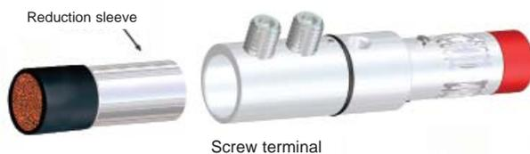
On set-screw contacts (up to 480amp power and 150 mm<sup>2</sup> cable sections), the cable is inserted into the set-screw terminal with the suitable reduction sleeve. Reduction sleeves are available for 25, 35, 50, 70, 95, 120 and 150 mm<sup>2</sup>. For all sleeve sizes, the stripping length is 33 mm (Pic. 1).
