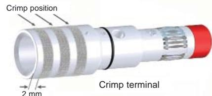
On crimp contacts (up to 750amp copper / 480amp bimetal, and up to up to 300 mm<sup>2</sup> cable sections), the position and number of cable compressions vary according to the different cable sections (see table below). Cable stripping length is 42 mm (Pic. 1).
