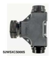
S2W with Syntax® SSX 19 pin connectors. On the S2W, the SSX 19 pin connectors can be with silver-plated or gold-plated contacts. Standard and reverse versions are available (standard version in the photo). The reverse version differs from the standard for the position where the input connector is assembled (on the reverse version, the input is inline with one of the outputs).
